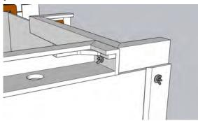
If required a bolt can be used to connect the 2 Pelmets (You would need to create your own hole)
