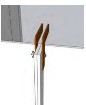
Start with fitting the MDF brackets using the bolts provided. Fit them by using the top connector on the rear of the wall. Remove the top bolt and fit the MDF using the new longer bolt.
