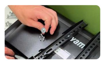
Each bracket is supplied with multiple size screws, select the correct size, add the washer and attach through the monitor arm, screwing into the back of the monitor.
