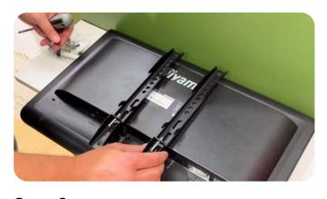
**Step 9**To fit the monitor arms, line the hole in the bracket arms with the holes on the back on your monitor.
