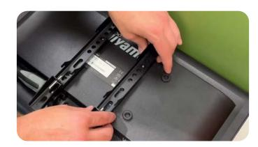
**Step 10**Place the black washers under the bracket arm to line up with the holes in the monitor.
